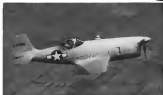
XP-77 Bell powered the XP-77 prototype with Ranger engine, armed it with 20-mm. cannon, two 50-cal. machineguns.
